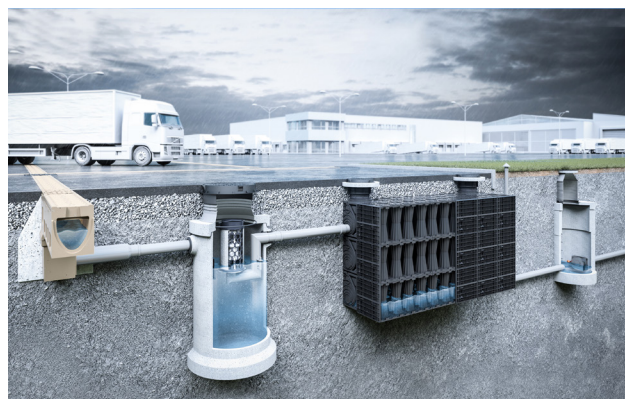
Sustainable management of surface water (Collect, Clean, Hold, Reuse)
